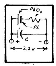
A cell can be represented by an *equivalent circuit*, illustrated by this diagram. The battery current encounters an internal resistance. The internal resistance depends not only on the material used but also the number of plates in each cell. The greater number of plates, the lower the internal resistance. With thin plates, SLI batteries have a much lower resistance that an EV battery with fewer thick plates. The parallel plates also act as a capacitor.
