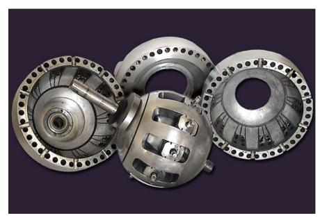
Typically, SGM machines have a large number of cylinders (from 12 to 36), which means smooth rotation, torque, and flows. There no peak loads on the parts. SGM produces no axial thrust; there is no need for thrust bearings on the main shaft, an advantage for hydraulic and other high-energy-density applications.
