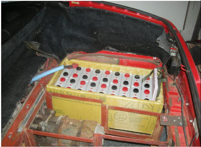
Rear trunk battery boxes made of Kevlar and polystyrene foam - per Jeff Miller
