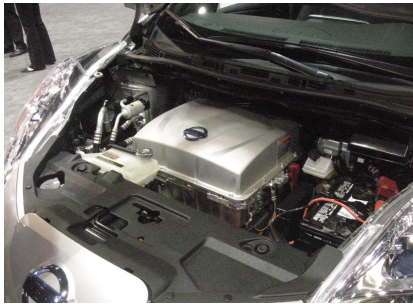
Nissan Leaf Inverter moved from trunk to top of motor providing more trunk space.
