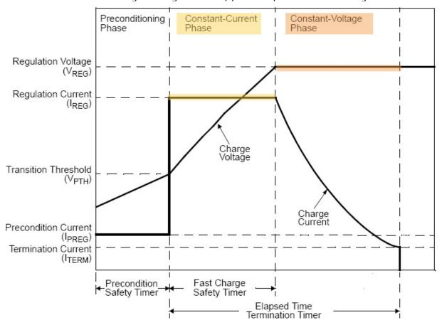
Constant-Current Phase: Charge rapidly at a high constant current (Ireg) until the voltage reaches Vreg.
