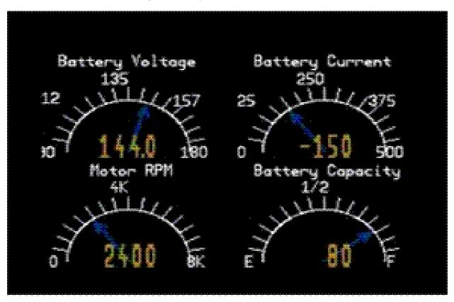
Obviously there are displays for Battery Voltage, Current, Tachometer and Battery Capacity. I was impressed that the little computer box also has a temp probe, as the battery temp is considered among the parameters used in calculating the Battery Capacity.
