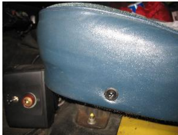
Perfect spot (as Jim suggested) to install high-low switch.
