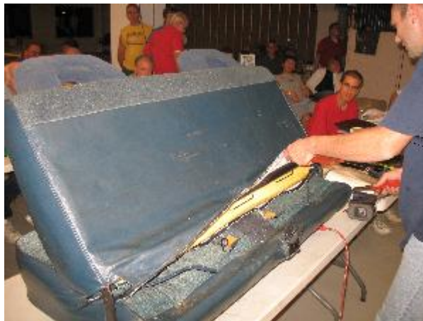
Jim begins by removing the hog rings holding the cover on.
