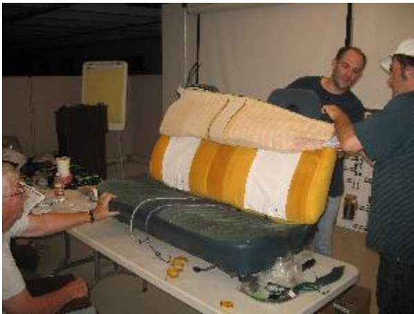
Upper heaters installed, put cover back on.
