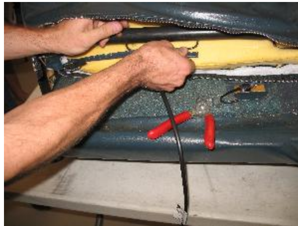
Reinstalling hog rings is easier with a special tool.
