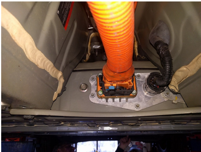
The primary ways the battery pack is electrically attached to the vehicle. The only other "connection" is a removable "safety plug" reachable from inside the vehicle which Bob had removed already before lifting up the vehicle.
