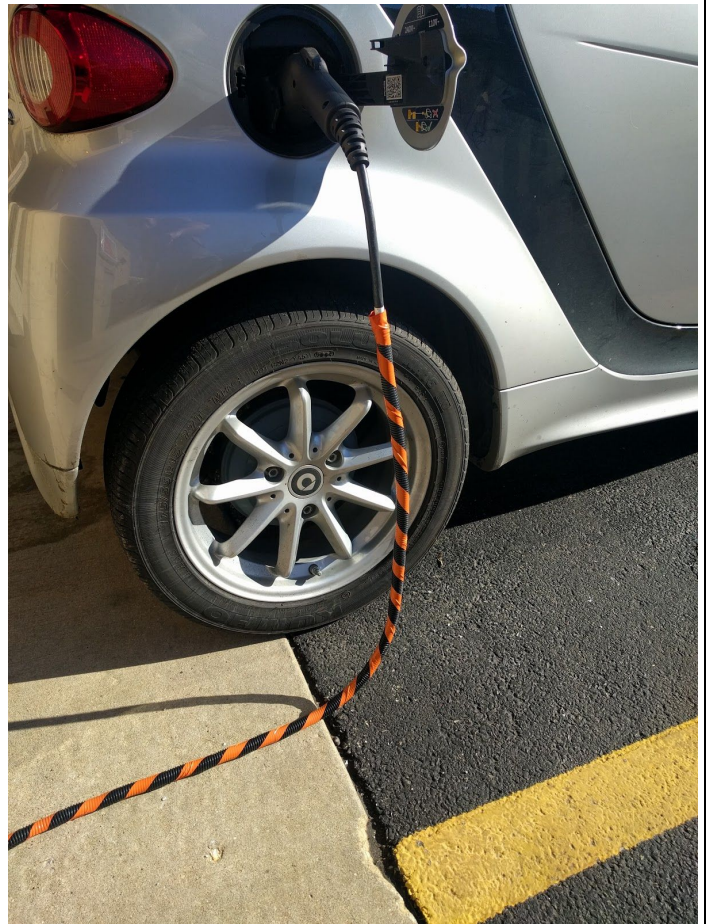
Fred getting a charge with Bob Baker's innovative charge cable where he used black tape on the orange cable to show "warning: high voltage!".
