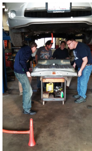
Success! Car lifted off and Battery wheeled out from underneath
