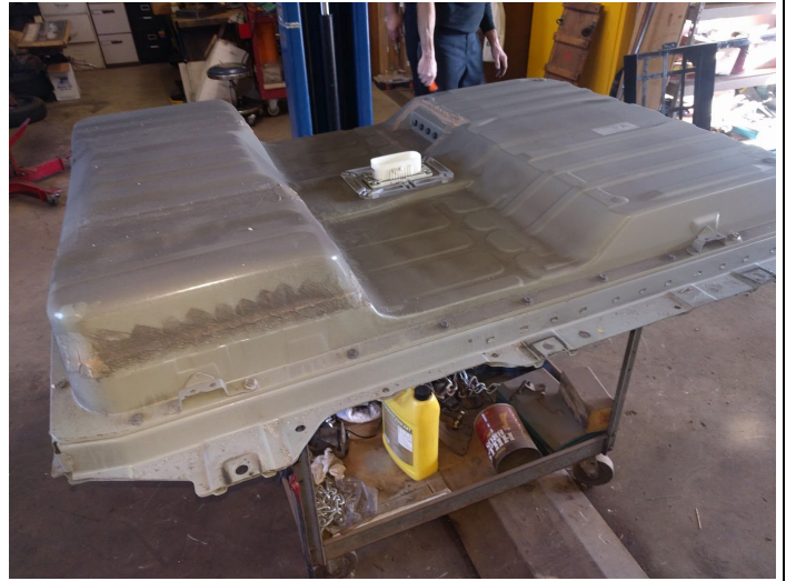
The cart was a great idea to hold and roll the battery pack from the lift into the vehicle for transport to the next location for analysis and repair. The white area in the top middle of the pack is where the previously mentioned "safety plug" mates.
