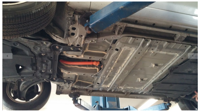
The Leaf was put up on the lift and undercarriage taken apart
